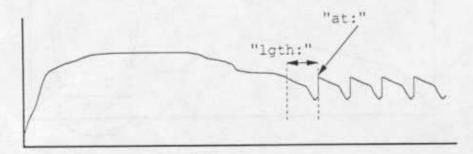
This is a poor choice of loop points. The sudden rise from the end of the loop to the beginning will cause audible "glitches"
