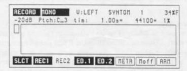
This page is the page where the actual recording takes place. Most of the parameters you can alter here are the same as the ones in the REC 1 page — from the position of the cursor when the page is first entered, they are:
