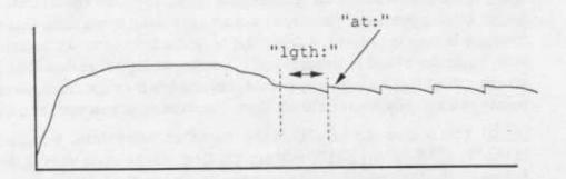
This is a much better choice of loop points. The rise from the end to the beginning will be less audible, and any "glitches" can be almost entirely eliminated using crossfading
