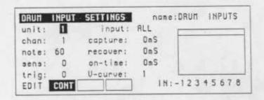
The name of the drum input settings may be altered using the NAME procedure. Either one of two ME-35Ts may be selected for parameter editing ("unit").
