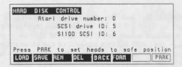
When using the IB-103 interface board, SCSI (Small Computer Systems Interface) numbers may be from 0 to 7, and the two numbers for the S1100 and the hard disk must be different. If an internal hard disk is fitted, the number of this hard disk will be set to 5, and the SCSI ID of the S1100 for use when accessing from an external initiator will be set to 6 (this number can be changed).
