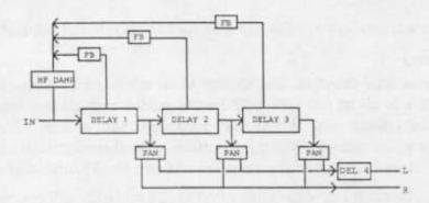
There are three delay lines that feed each other in series. Delays 1 - 3 are capable of up 360mS of delay whilst delay 4 is capable of 180mS of delay and, in total, you have 1260mS of delay. Each delay has its own feedback loop and pan position control and repeat echoes have the effect of 'flying' round the stereo image. These parameters allow you to create a wide range of echo effects that emulate the warmth and density of tape delay units with their complex, multi-head echoes.
