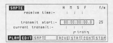
The receive time field shows the current time being fed to the timecode reader from an external source. It will also detect the frame rate used on the external source and this is displayed underneath the f/s field shown in the top right hand corner of the screen.
